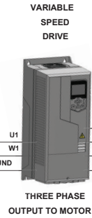
SINGLE PHASE TO THREE PHASE WIRING DIAGRAM
